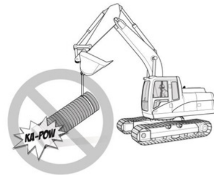
FIGURE 3 - LIFTING LARGE DIAMETER PIPE
