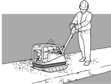
Vibratory plate equipment – Used for non-cohesive backfill material.
