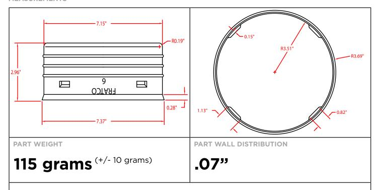
These specifications are held in standard according to ASTM F667 - Standard Specification for Polyethylene Plastics Pipe and Fittings material.
