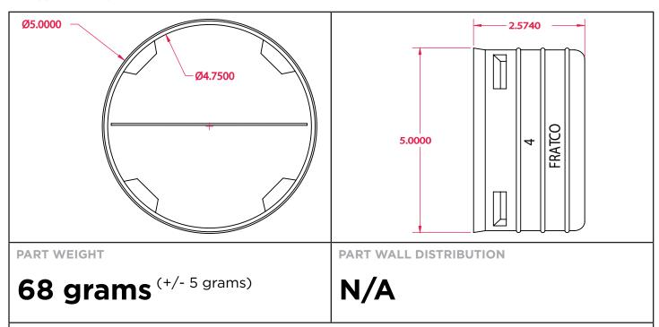
These specifications are held in standard according to ASTM D3350 - Standard Specification for Polyethylene Plastics Pipe and Fittings material.
