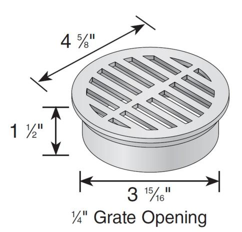
Part #: 11, 12, 13 and 13S Material: (HDP) High Density Polypropylene Color: #11(Black), #12(Gray), #13(Green), & #13S(Sand) Fits: 4" sewer and drain pipe & fittings, 4" corrugated and triple wall pipe. Grate Opening: 1/4" Open Surface Area: 3.85 Sq. Inches Head Pressure / Flow Rate: Head (inches) - Max Flow 1"= 16.66 GPM 0.5" = 11.78 GPMWeigh Per Each: 0.16 lbs. UV inhibitor
